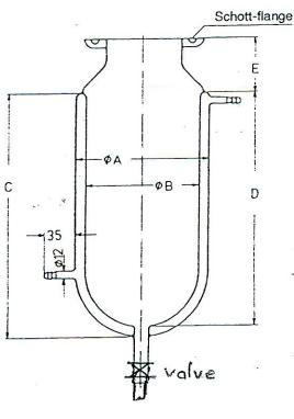
Jacketed Reaction Vessel Capacity = 2000 ml.
