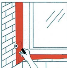
Picture 3: Remove protective foil on the butyl side, adhere the tape to the surface and press on carefully.
