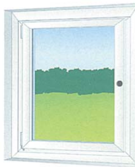
Picture 4: The connecting joint can be covered visually with a flat rail.
