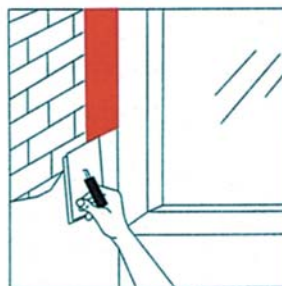
Picture 4: The fleece-lined side can be plastered or painted with dispersion paint.
