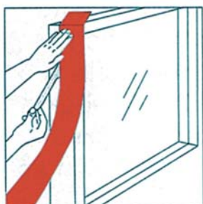
Picture 1: Press adhesive strip of fleece-lined side carefully onto the window frame.
