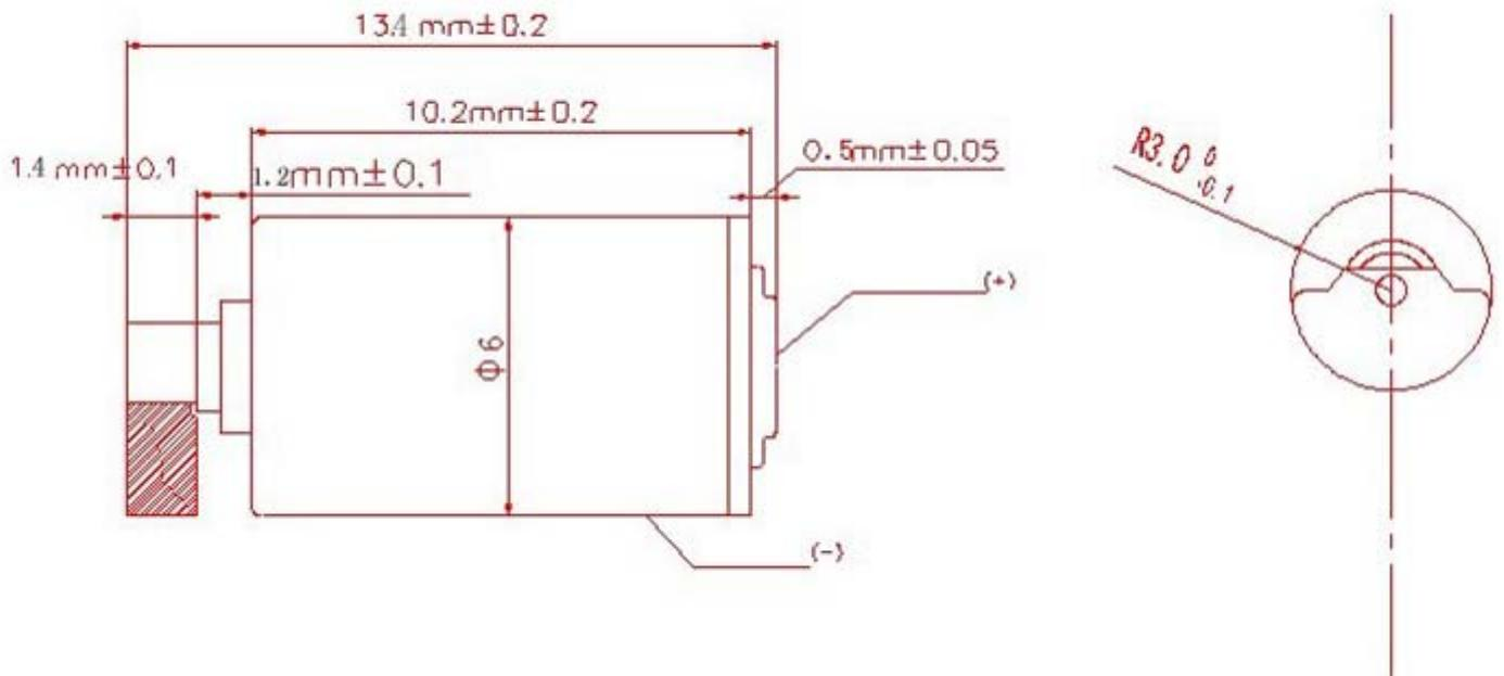
Figure 1 Motor Housing Configuration
