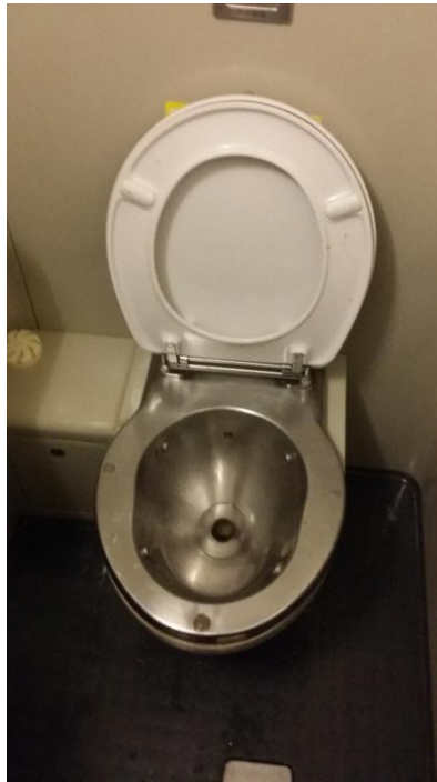
Photo 1 – A Stainless Steel Toilet Bowl in an EMU
