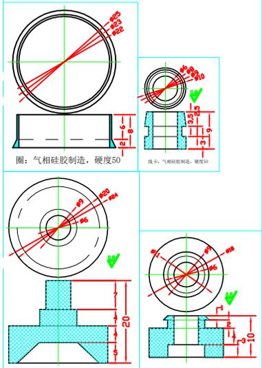
圈：气相硅胶制造，硬度50
